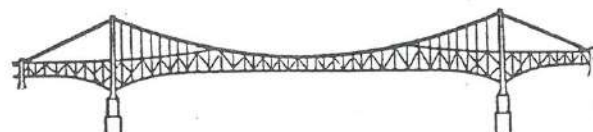
(i) FLORIANOPOLIS TYPE CONTINUOUS PAST TOWERS (Proposed for Sydney, N.S.W., 1923)
